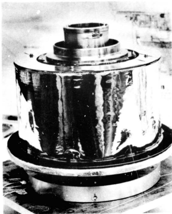
Fig. 3 The HELIOS despin drive assembly
