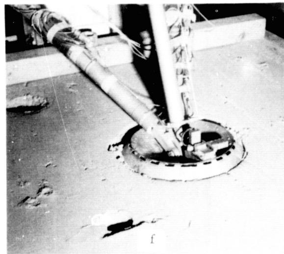
Figure 3 - Footpad Soil Penetration Tests
